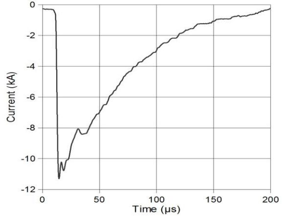
Fig. 1. Return stroke type ICC-pulse in GBT flash #759
