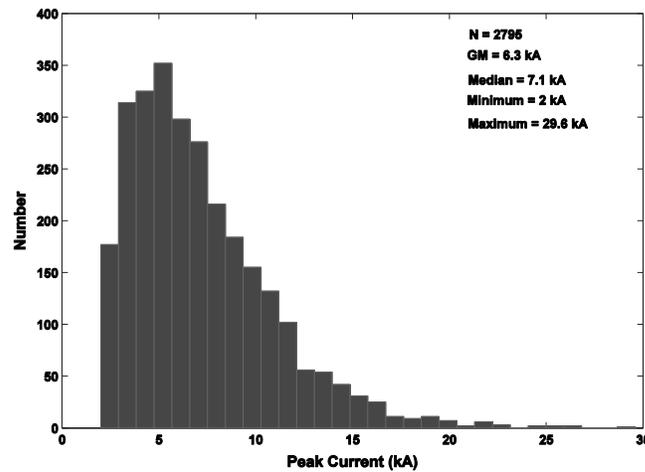
**Figure 4.** Peak current distribution of pulses associated with upward negative flashes measured at the Säntis Tower.
