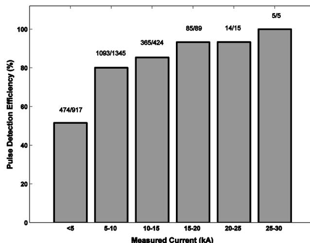
**Figure 5.** EUCLID detection efficiency as a function of pulse peak current measured at Säntis (the bin size of 5 kA) for upward negative events.
