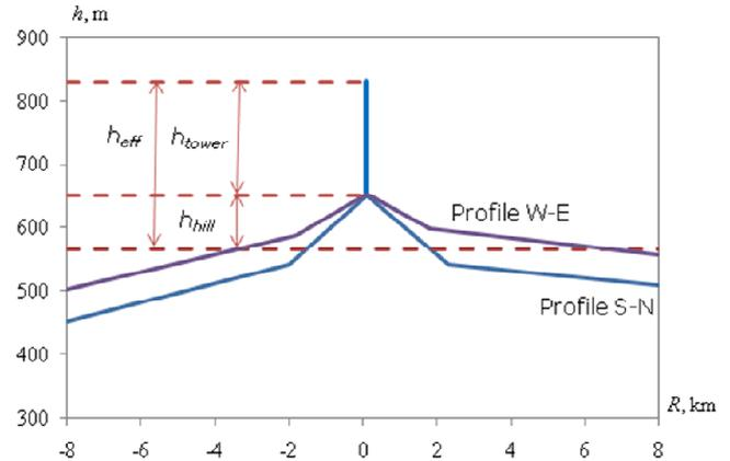
Figure 5. Illustration of the estimation of the effective height.
