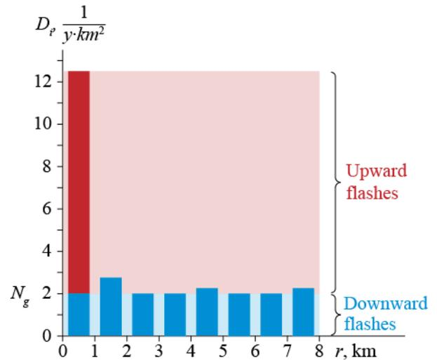
Figure 3. The lightning flash density within each ring, the tower is situated in the first one.
