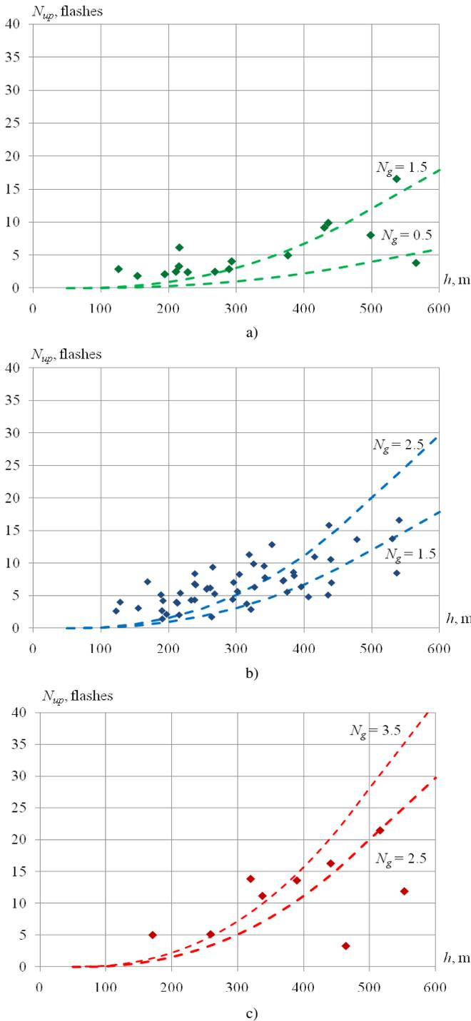
Figure 6. Number of upward flashes from the structures of different height situated in the regions with a)  $N_g = 0.5-1.5$ , b)  $N_g = 1.5-2.5$ , c)  $N_g = 2.5-3.5$  flashes $\cdot$ km $^{-2}\cdot$ y $^{-1}$ . In each figure, we have also presented the results obtained using Eriksson's formula for the corresponding values of  $N_g$ .
