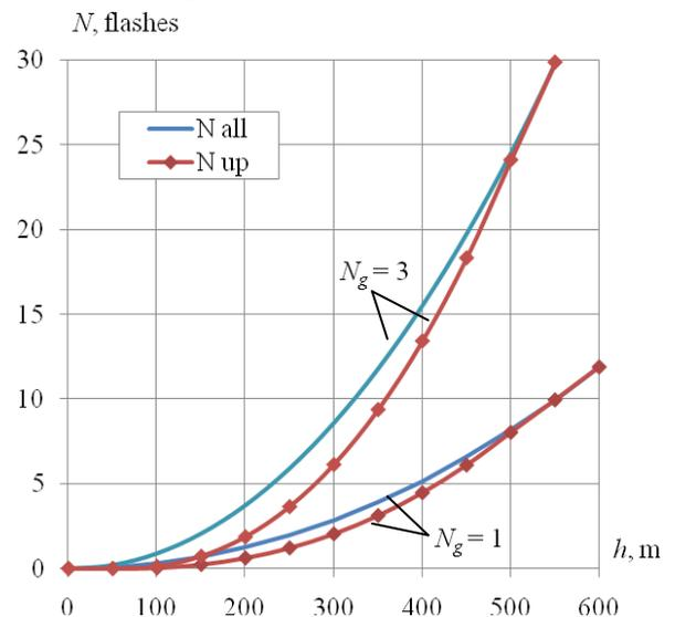
Figure 1. Variation of the total number of flashes and the upward flashes as a function of the structure height  $h$  and considering two values of ground flash density  $N_g$ , based on equations (1)-(3).
