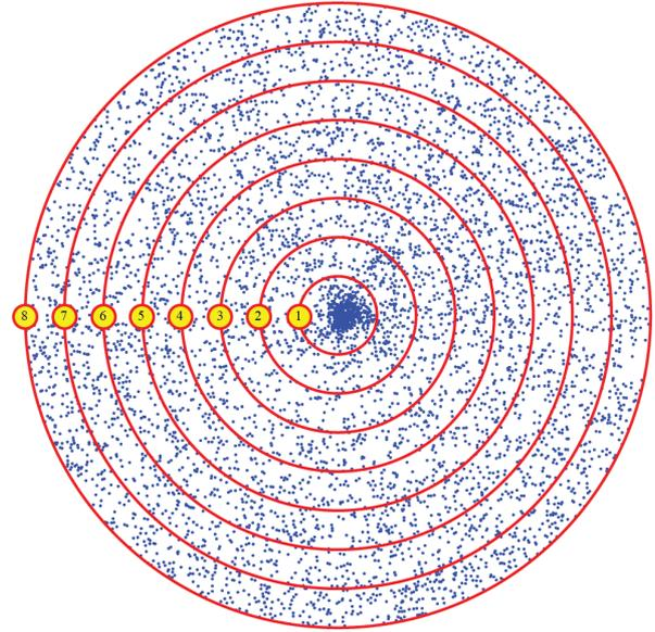
Figure 2. Lightning flashes detected during ten years within the circle of 8 km around a tower situated in the center.
